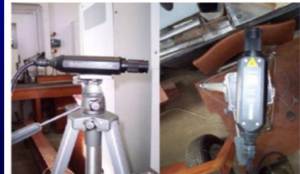
Figure 35 – Single Point Laser Vibrometer by Polytech
